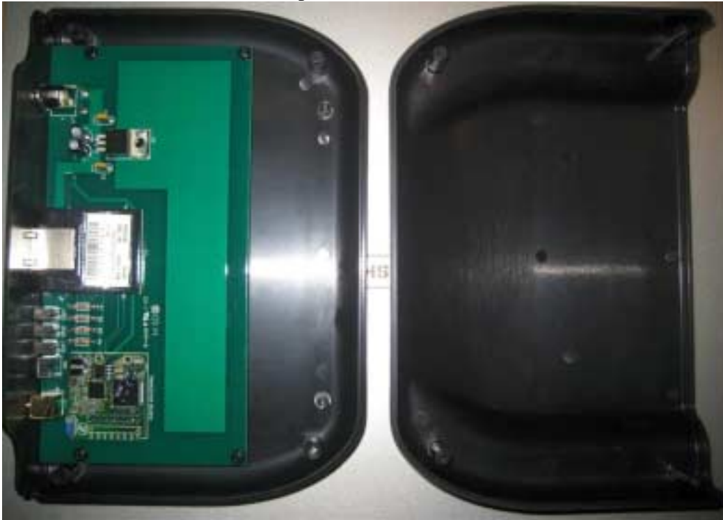
Base Station Inside & PCB Components Side View
