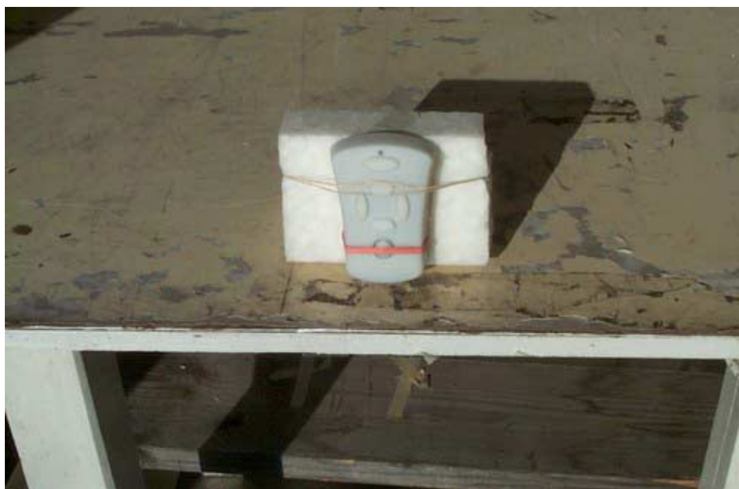
Figure 3.4 Radiated Test Setup – Z axis
