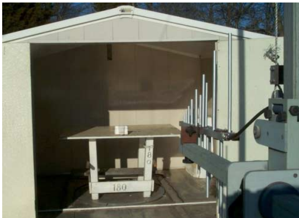
Figure 3.1 Radiated Test Setup
