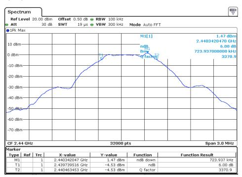
Modulation Standard: GFSK Channel: 19
