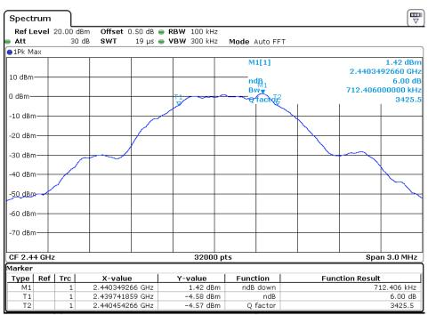
Modulation Standard: GFSK Channel: 19
