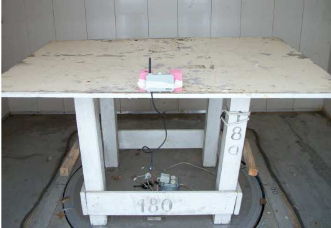
Figure 3.1 Radiated Test Setup
