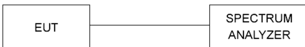
Figure 1 - Bandwidth Measurements Test Setup
