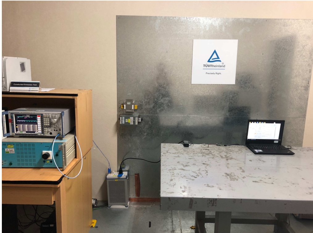
Photograph 6: Set-up for for Mains Conducted testing Front
