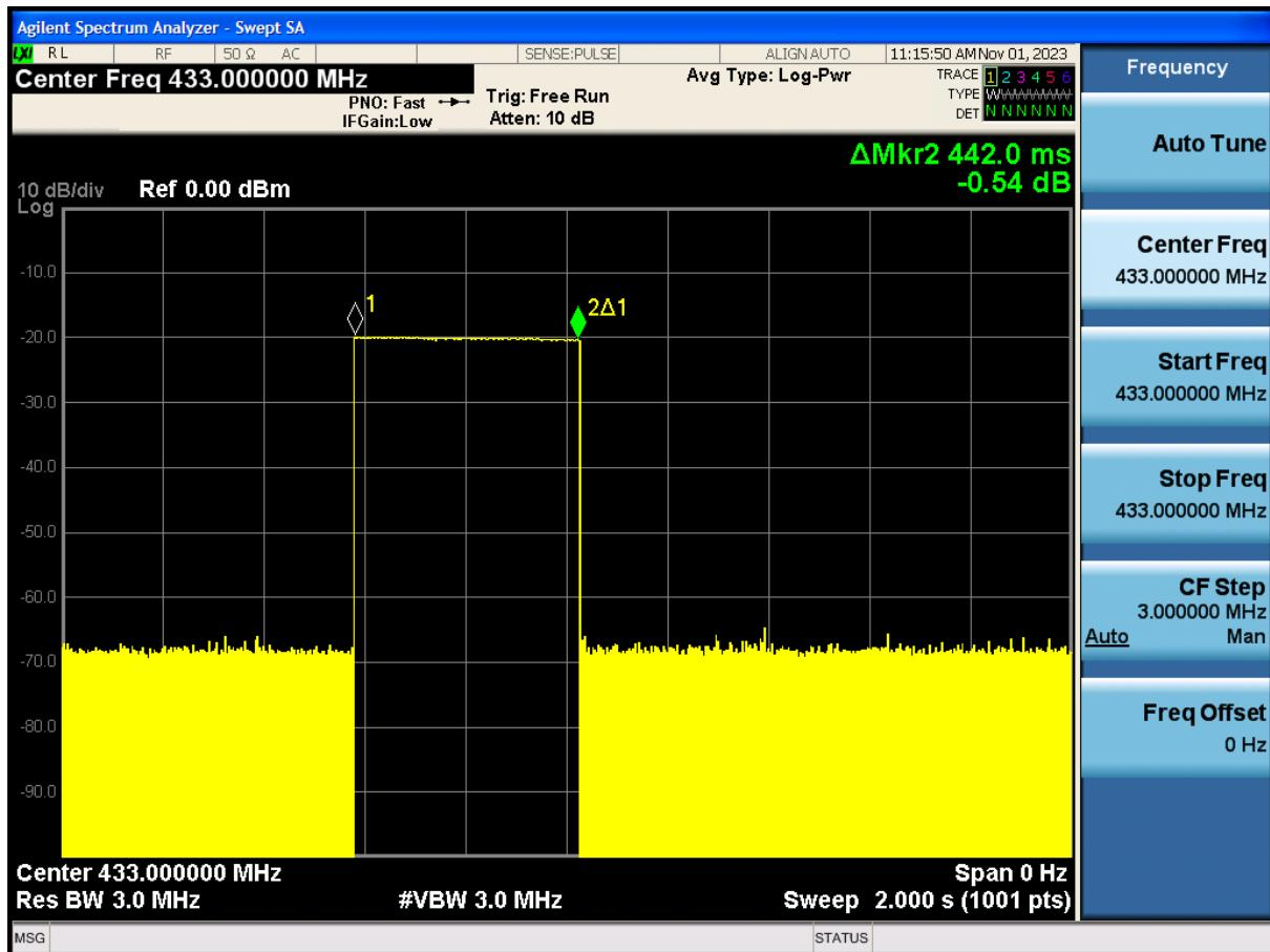
Result: Pass, the EUT had automatically deactivated transmission within 5 seconds.
