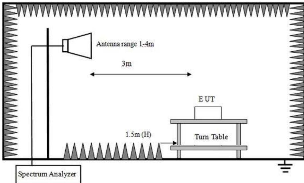
Above 1GHz Test Setup
