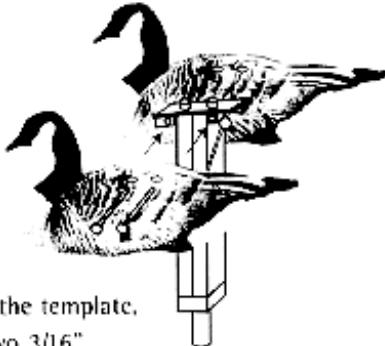
Using the template, drill two 3/16" holes in each side of the decoy, as shown. Insert the bolt from the outside of one decoy half, thru the mechanism and the other half of the decoy. Secure with nut.
