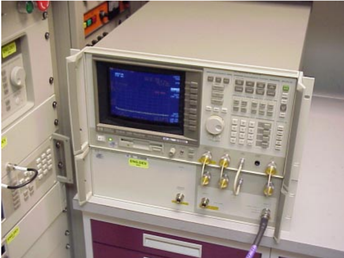
Figure 12.4 HP8546A EMI Receiver, No Filter
