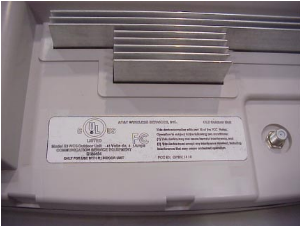
Figure 5.4 Close-up of Label on R3 WCS Outdoor Unit
