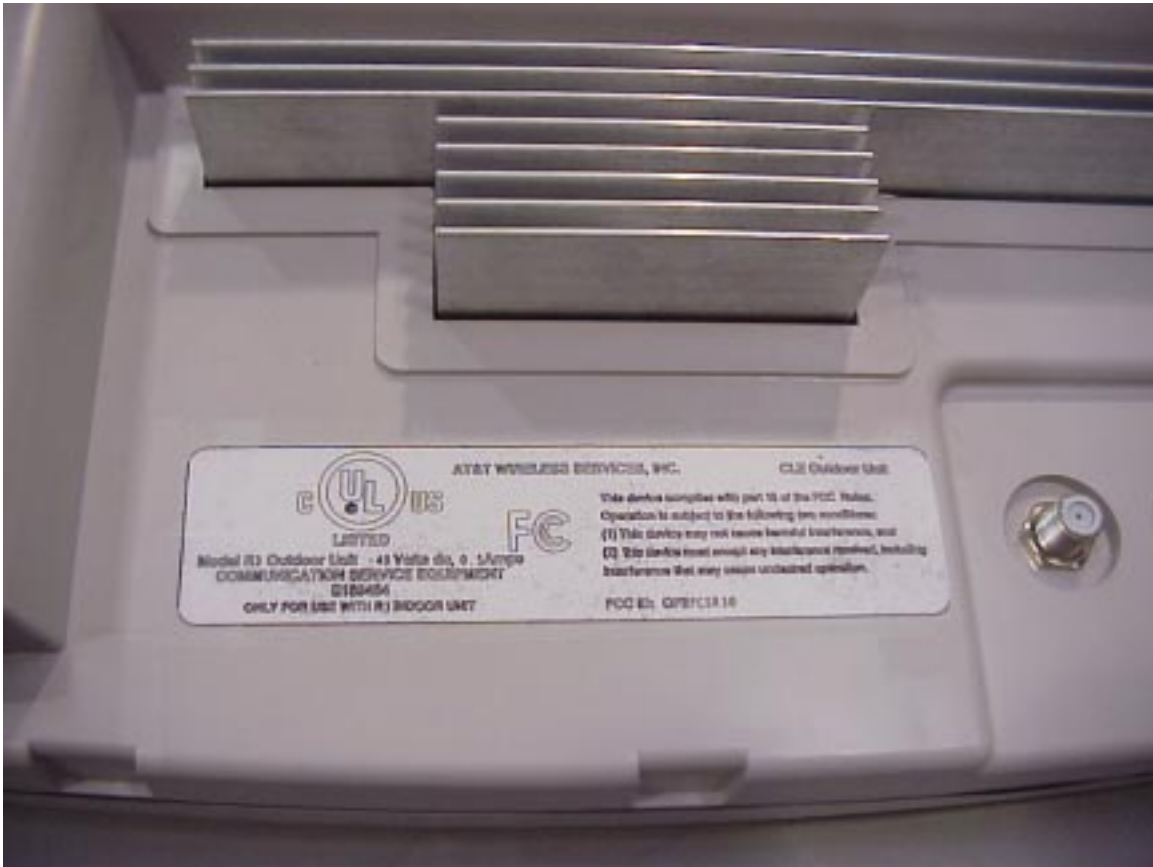
Figure 5.4 Close-up of Label on R3 Outdoor Unit
