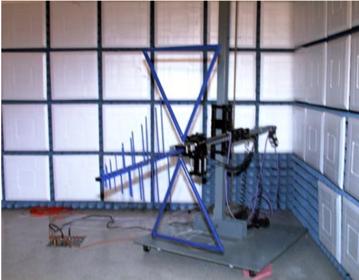
Figure 12.13 Radiated Emission 30MHz - 1GHz Test Setup
