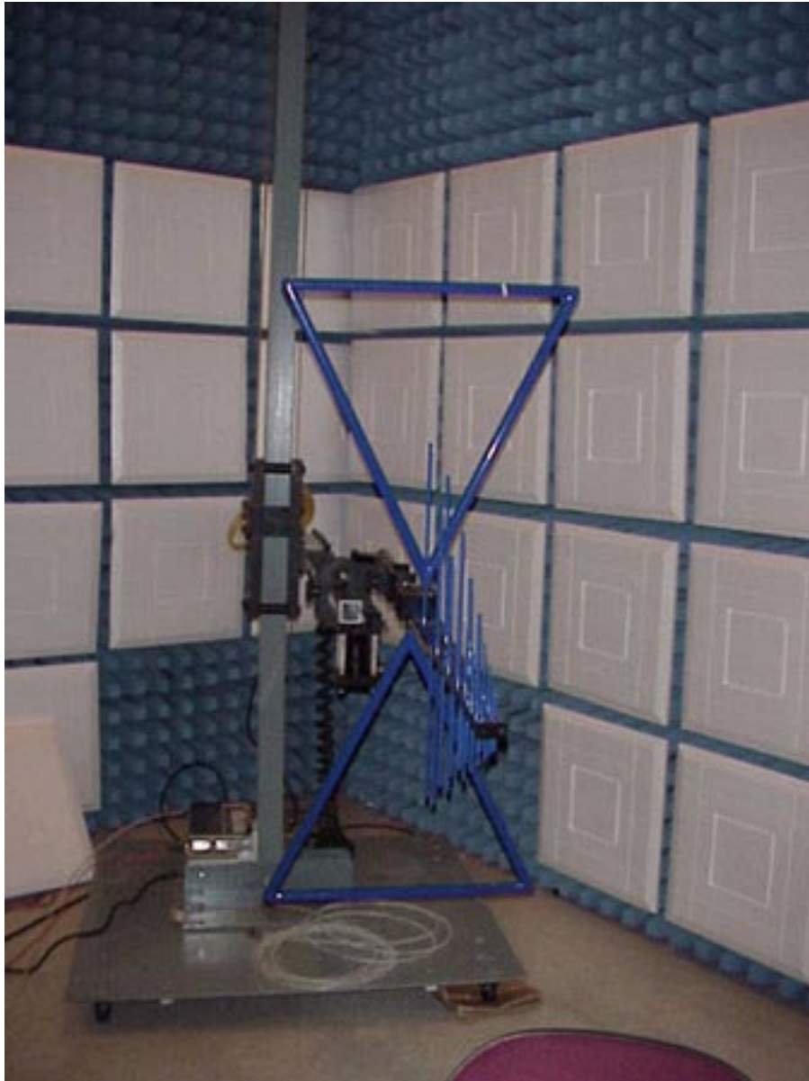
Figure 12.14 Radiated Emission 30MHz - 1GHz test set-up
