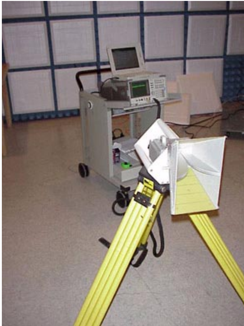
Figure 12.13 HP 84300A E62 Microwave Intentional Radiator System
