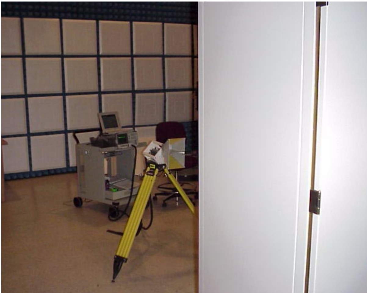
Figure 12.12 HP 84300A E62 Microwave Intentional Radiator System
