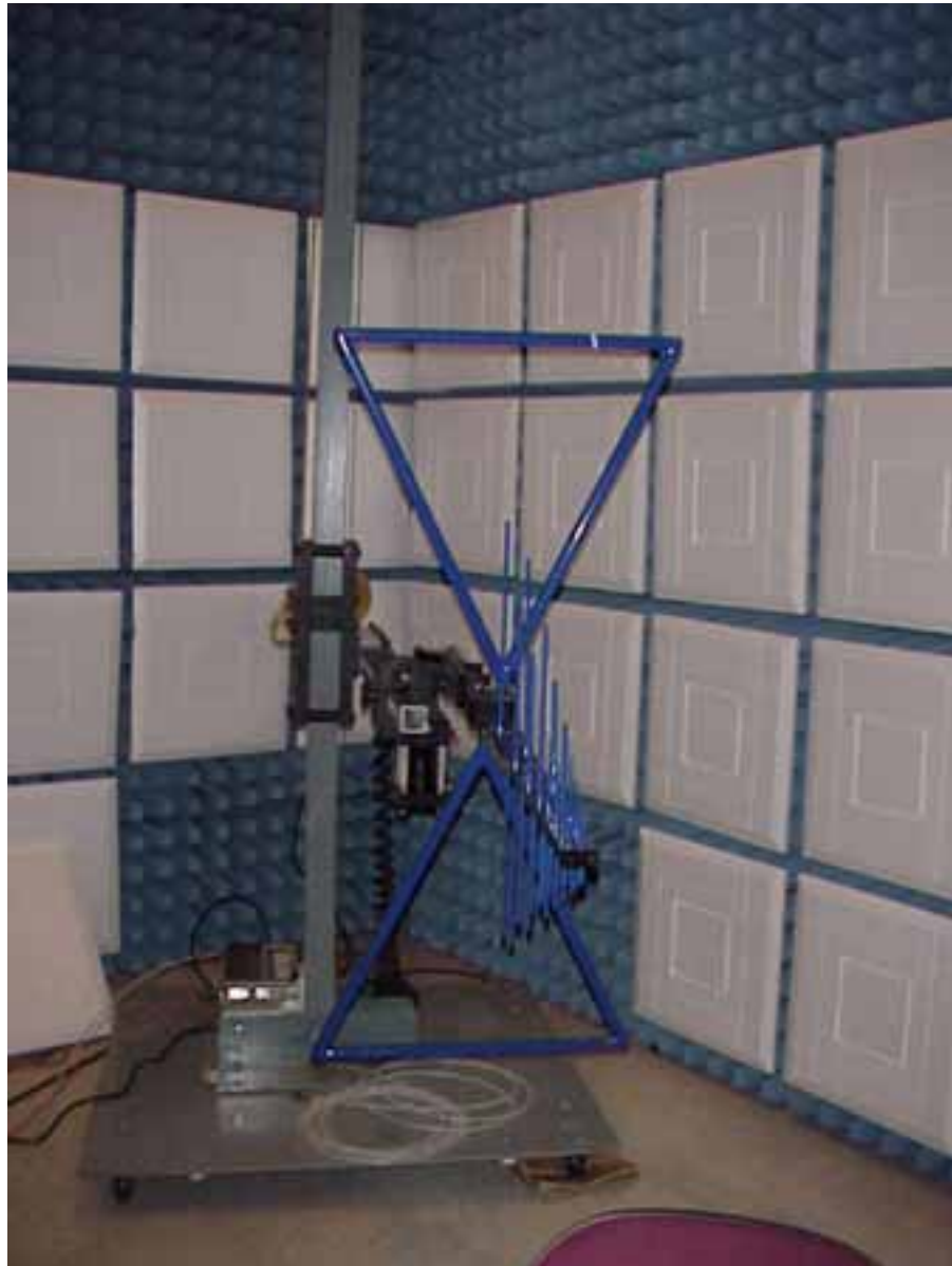
Figure 12.14—Radiated Emission 30MHz - 1GHz test set-up
