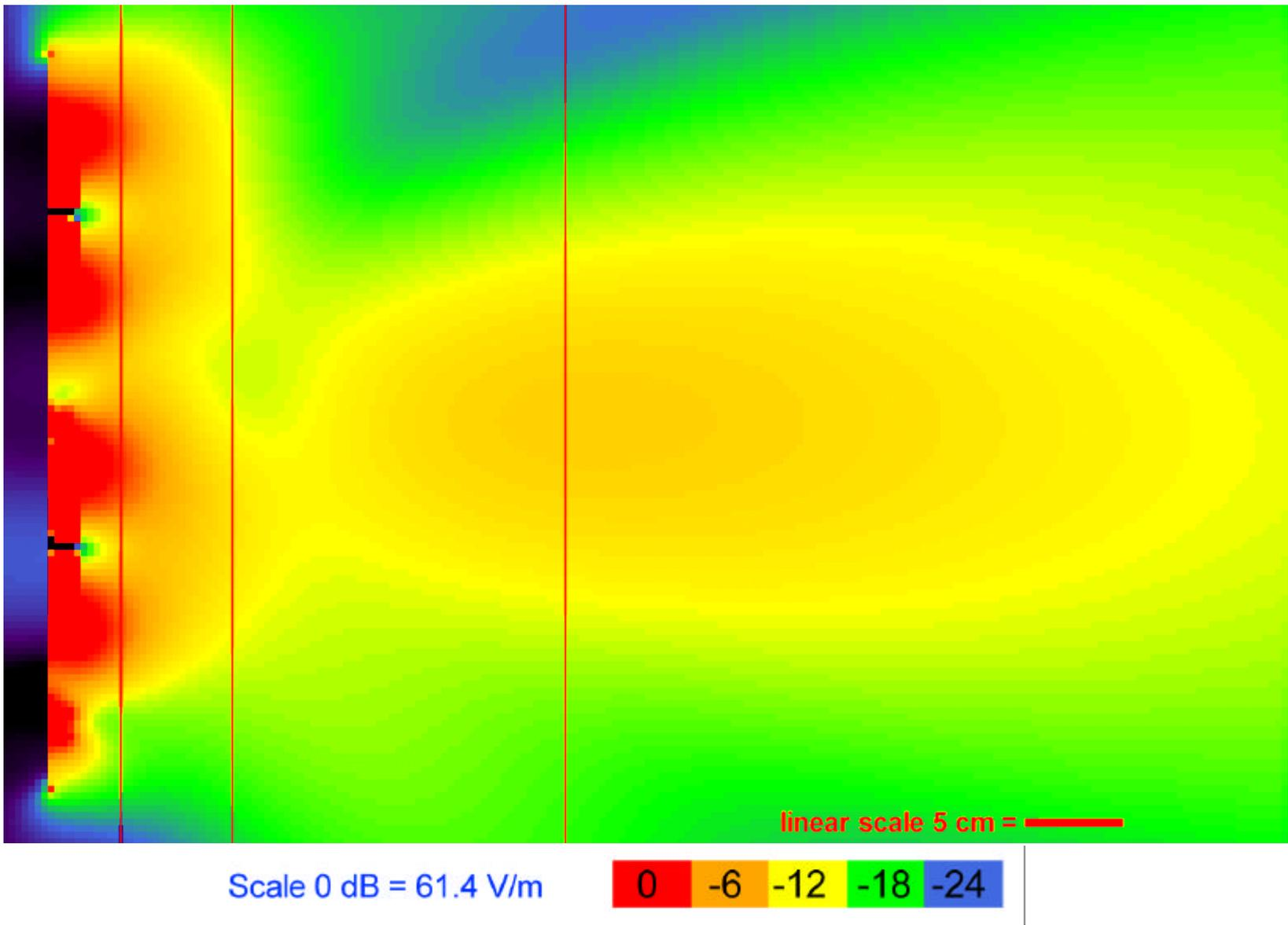
Figure 5.17. FDTD derived E-field of AT&T RU antenna in x-y plane compared to ANSI/IEEE exposure standard (Scan D, vertical plane through middle of right row of patches).
