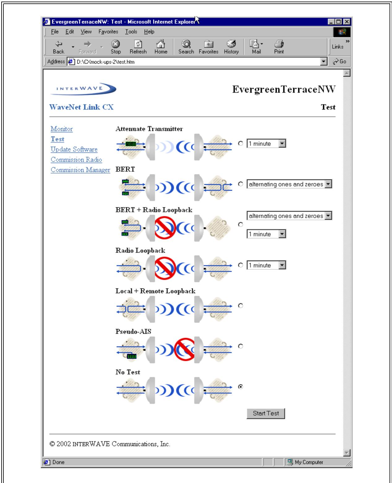
Figure 4-6 Link CX Test Web Page
