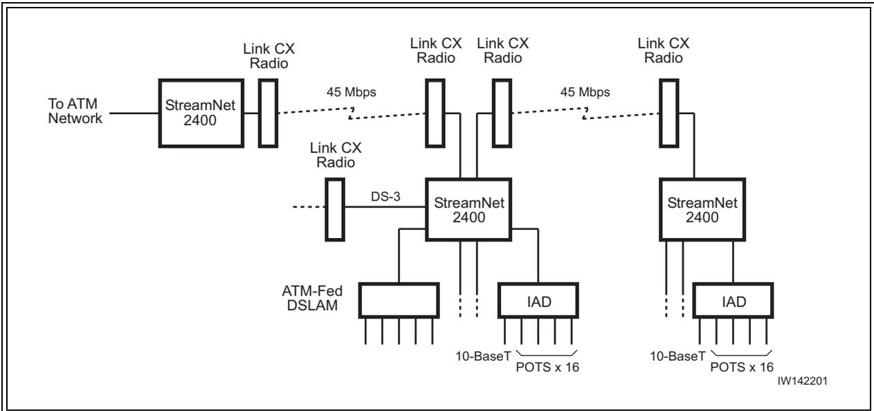
**Figure 1-6** Typical Wireless MTU/MDU Access Configuration
