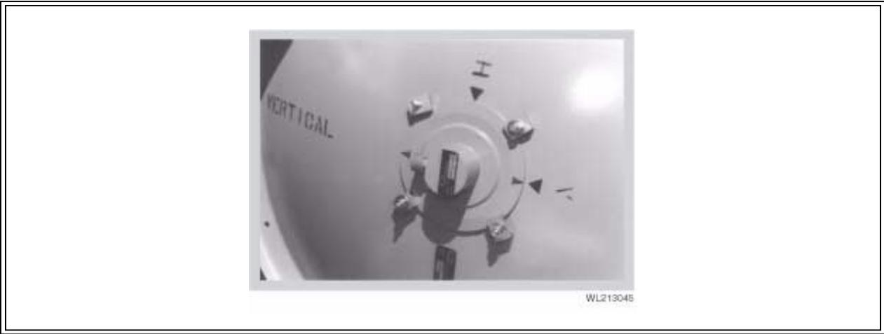
**Figure 4-27** Feed Horn Installation for Vertical Polarized Operation
