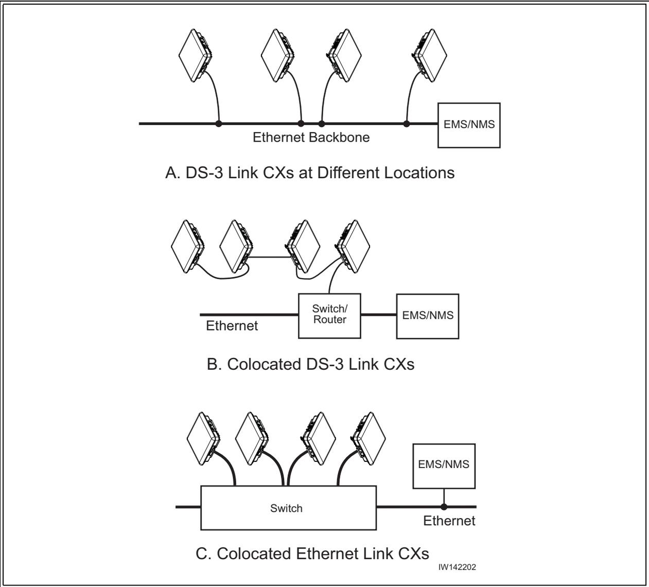
**Figure 3-3** Typical EMS/NMS Ethernet Connections
