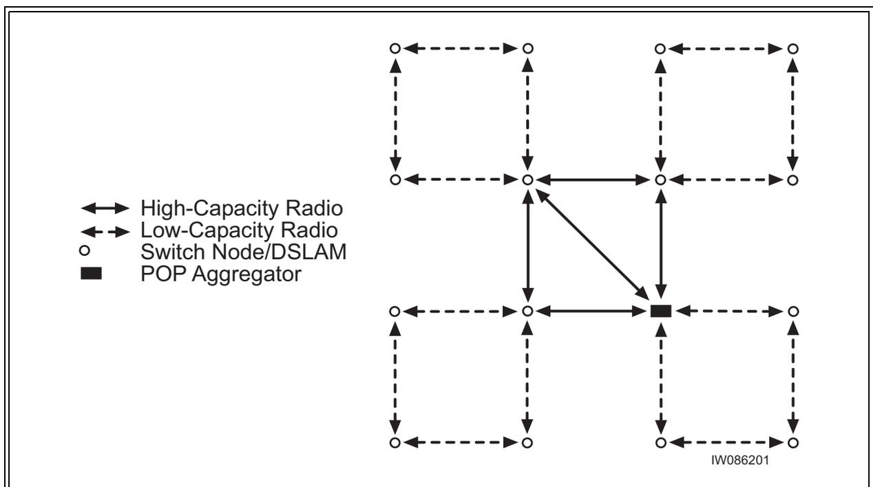
**Figure 1-7** Typical Wireless DSLAM Mesh Backhaul Network
