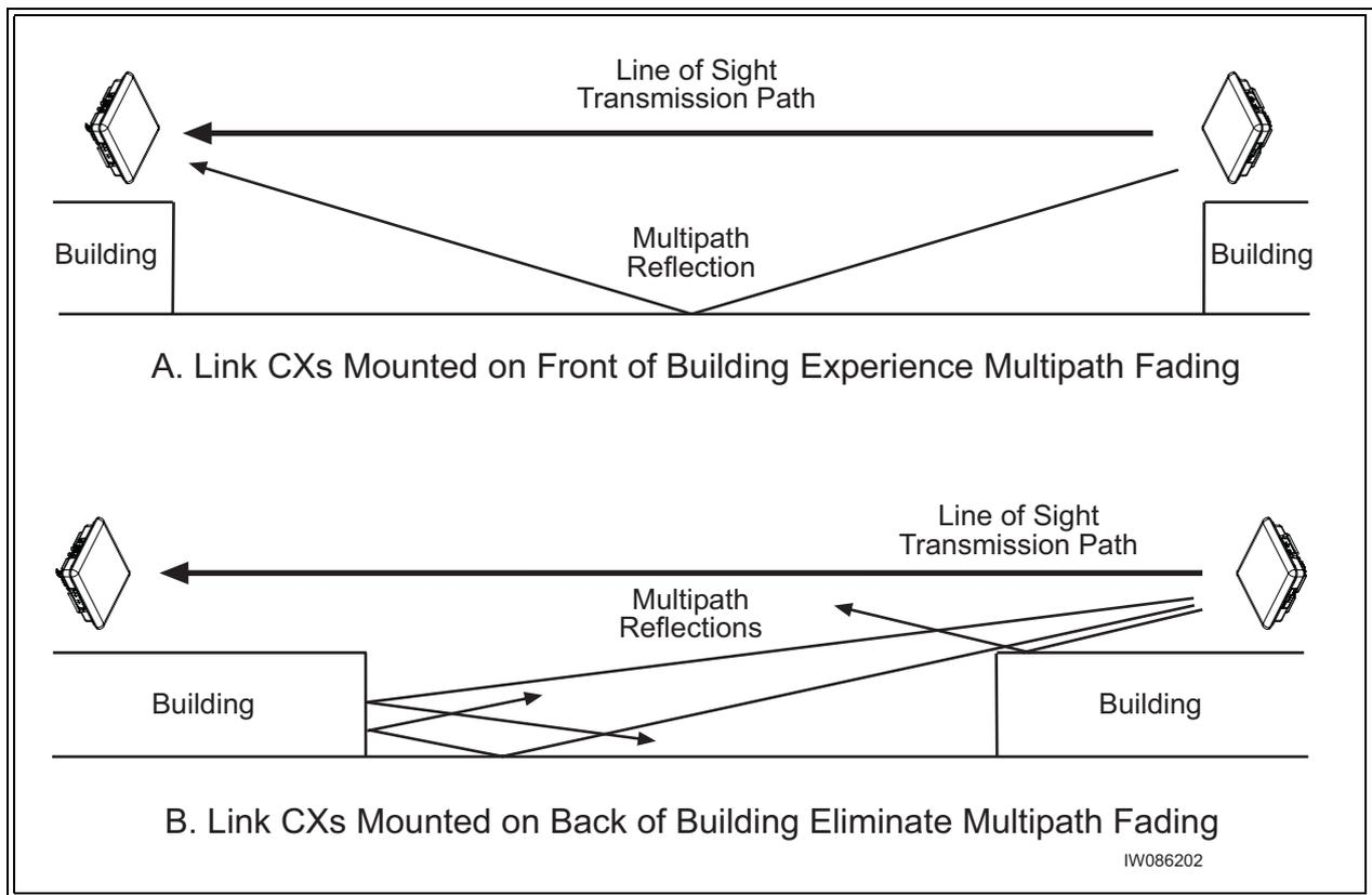
**Figure 3-2** Preventing Multipath Fading from Ground-Level Surfaces
