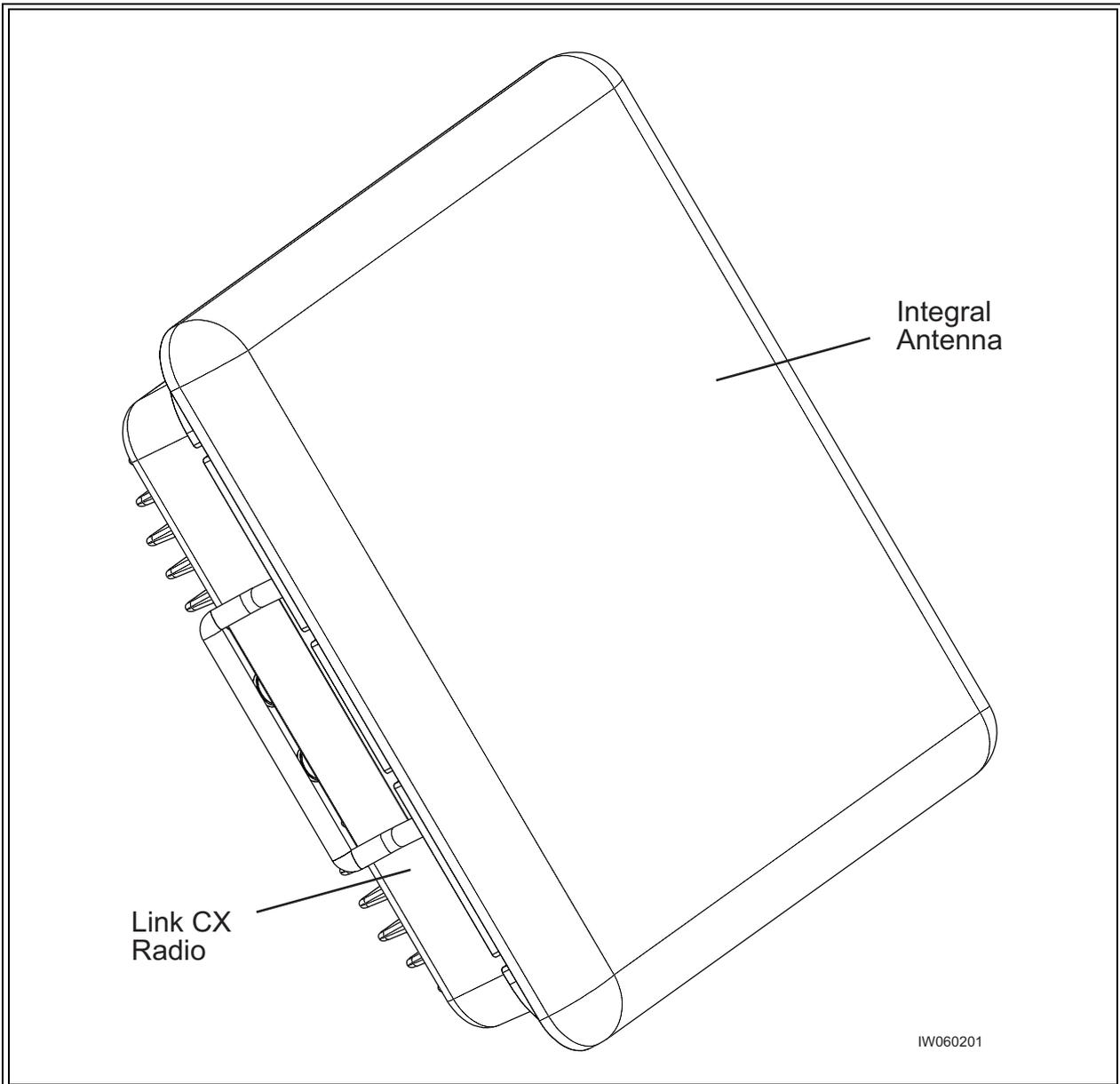
**Figure 1-4** Integral Antenna and Link CX Radio
