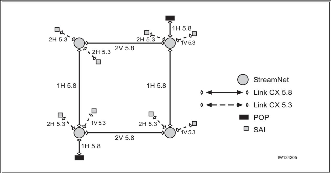
**Figure 1-8** Typical Wireless ATM Mesh Backhaul Network
