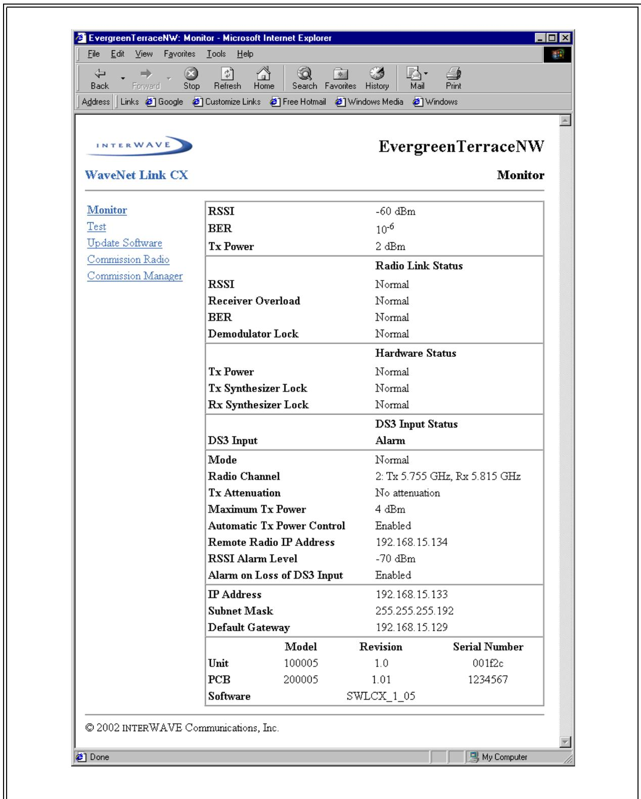
**Figure 4-3** Typical 5.8 GHz Link CX Monitor Web Page
