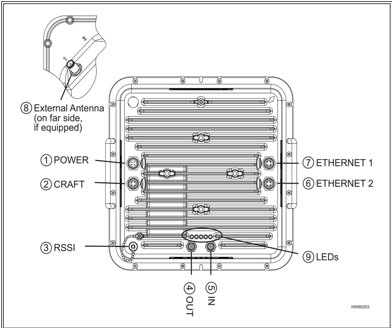
**Figure 1-3** Link CX Interface Connectors and Indicators
