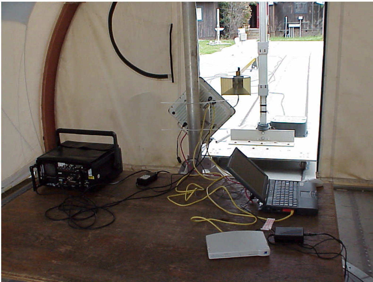
Link CX, 15.205 Radiated emissions, Restricted bands, setup
