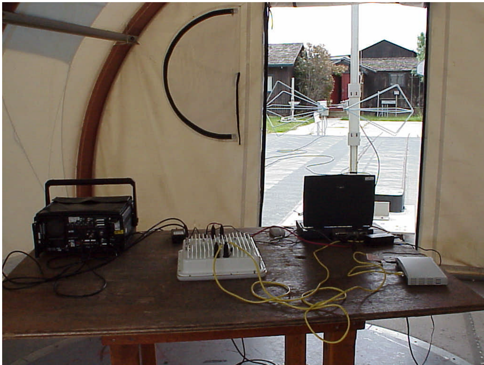
Link CX, 15.209 radiated measurement setup, 30 MHz to 1 GHz
