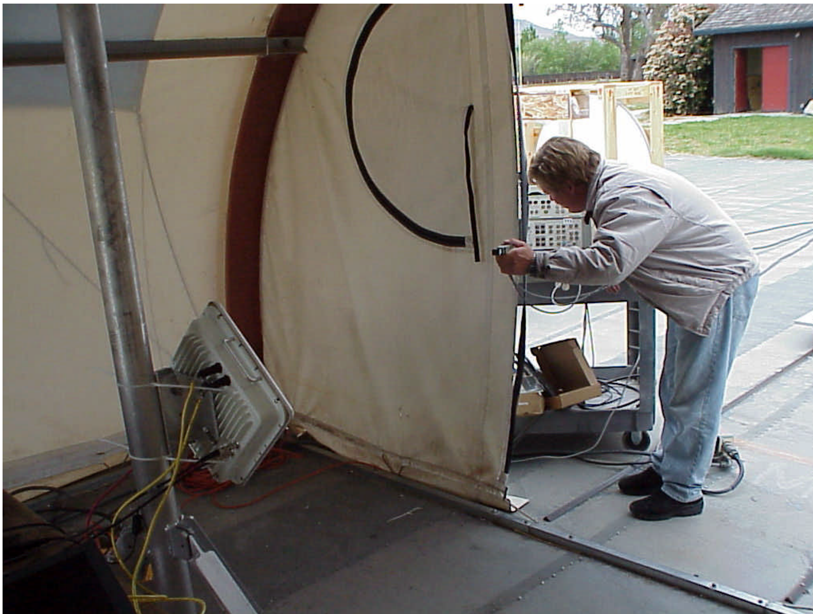
Link CX, 15.205 Radiated emissions, Restricted bands, setup
