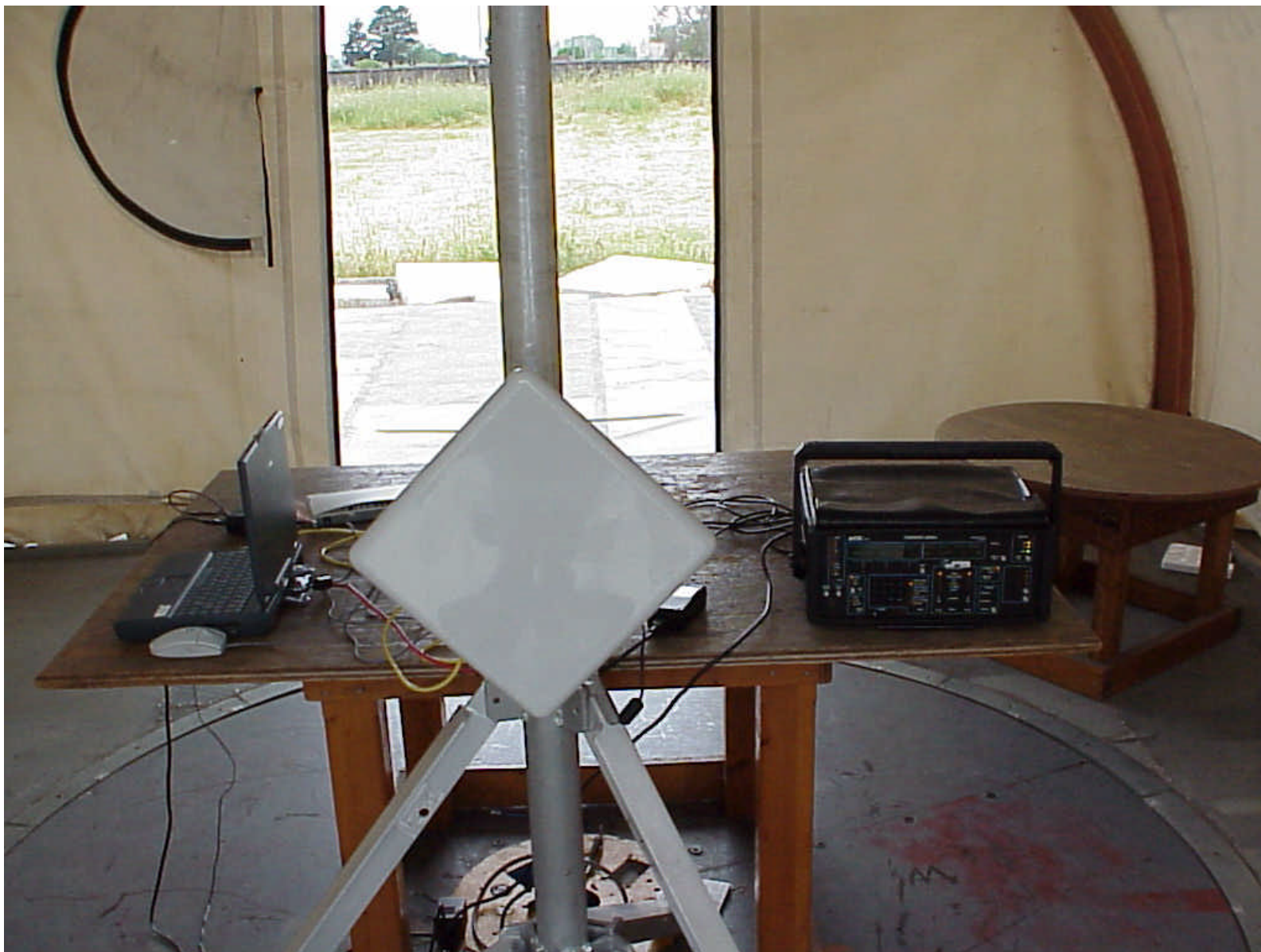
Link CX, 15.205 Radiated emissions, Restricted bands, setup
