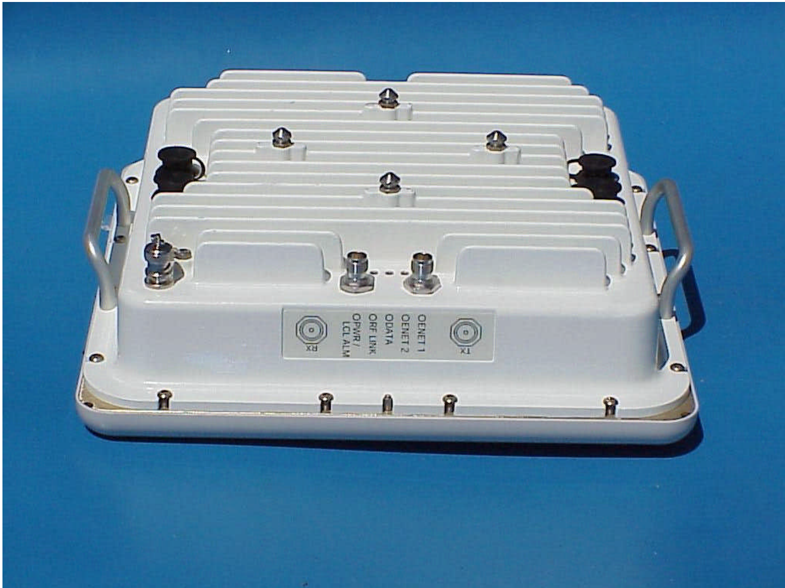
Link CX external side view showing DS3 connectors and LED windows
