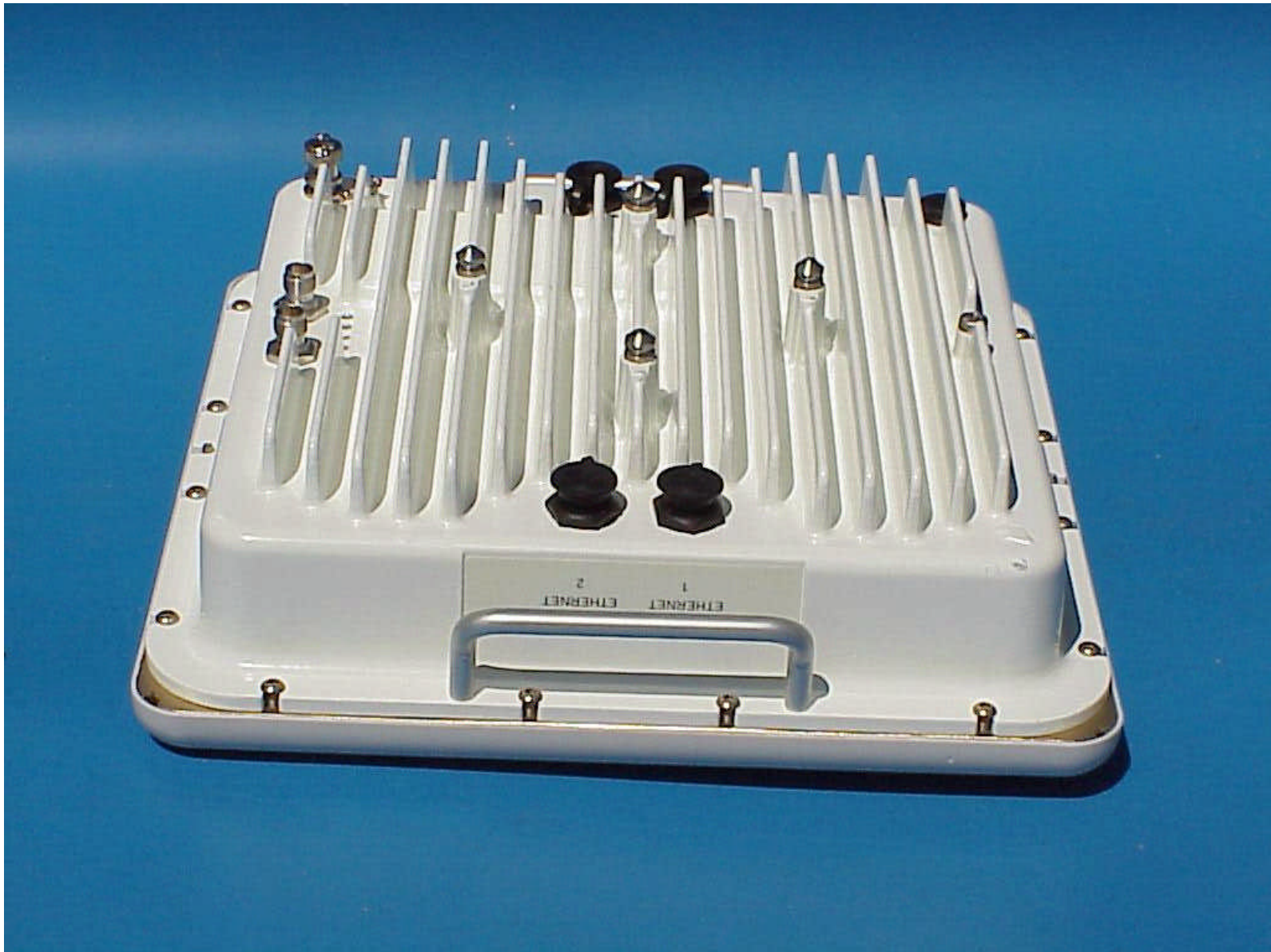
Link CX external side view showing 10 / 100 base-T connectors
