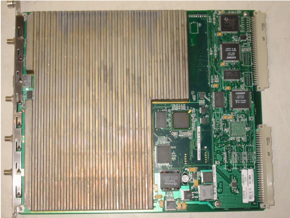
TRX Assembly, shield over board
