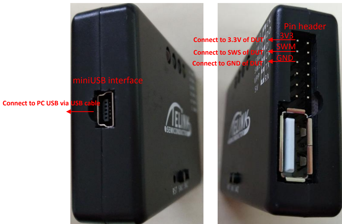
Figure 3 Connection chart 1 to download FW into DUT via TLR8266BR56
