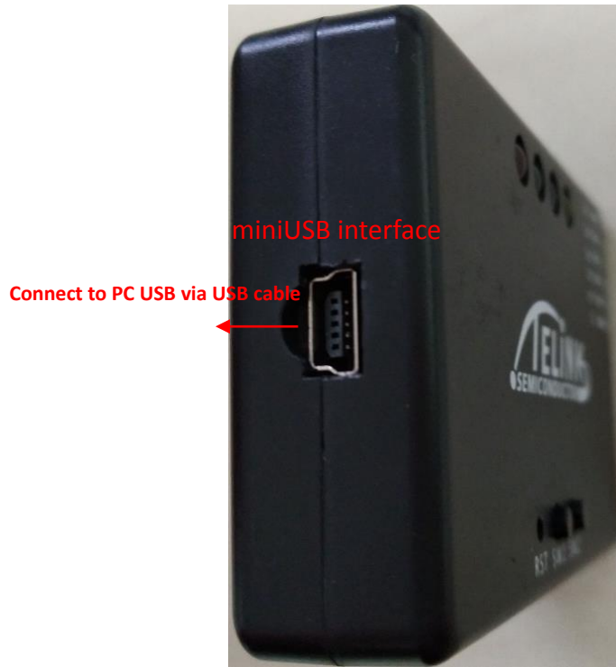
Figure 2 Connection chart to supply power for TLSR8266BR56
