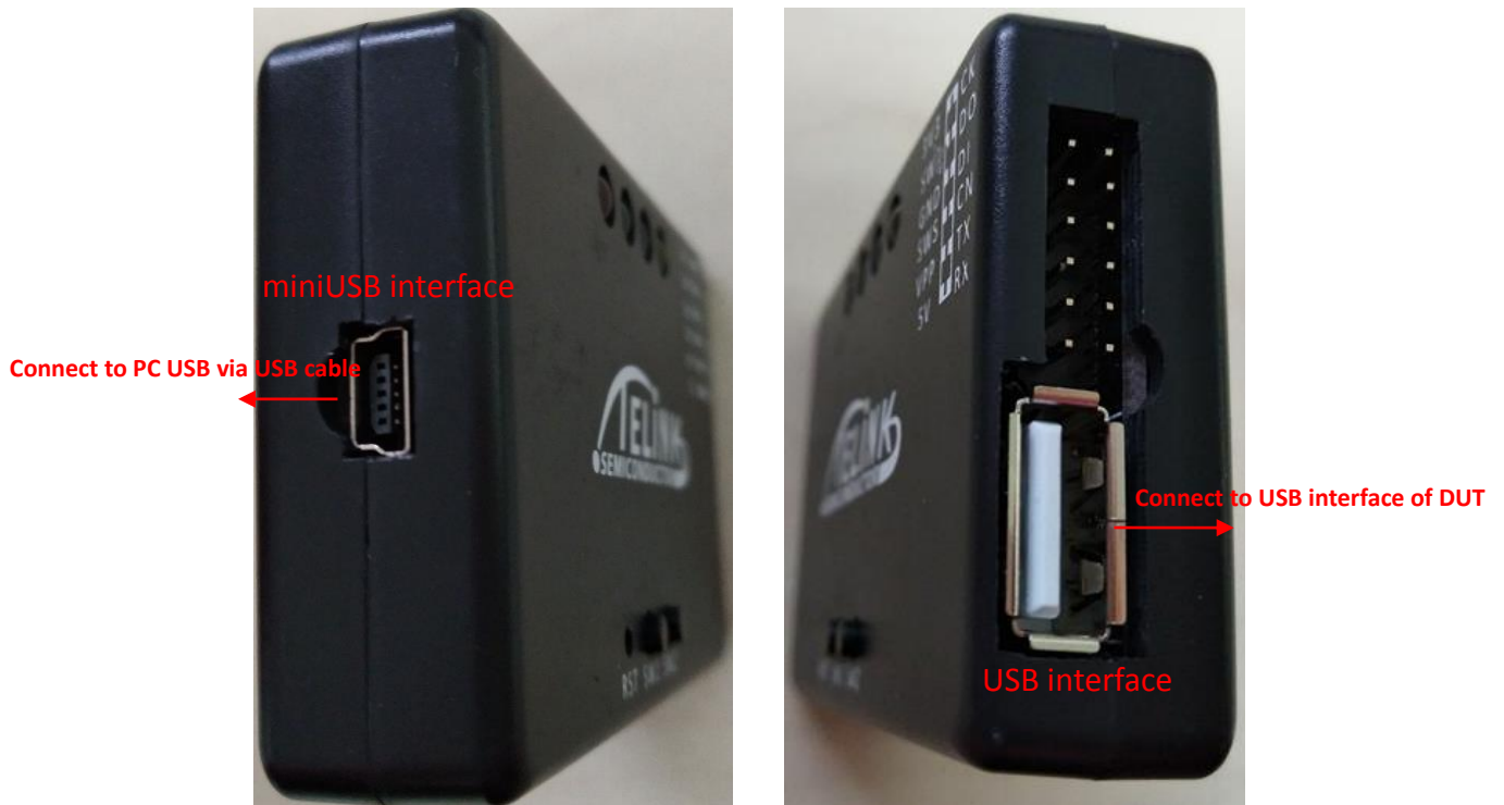
Figure 4 Connection chart 2 to download FW into DUT via TLSR8266BR56
