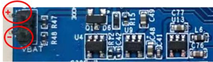
Figure 2-3 Battery power supply
