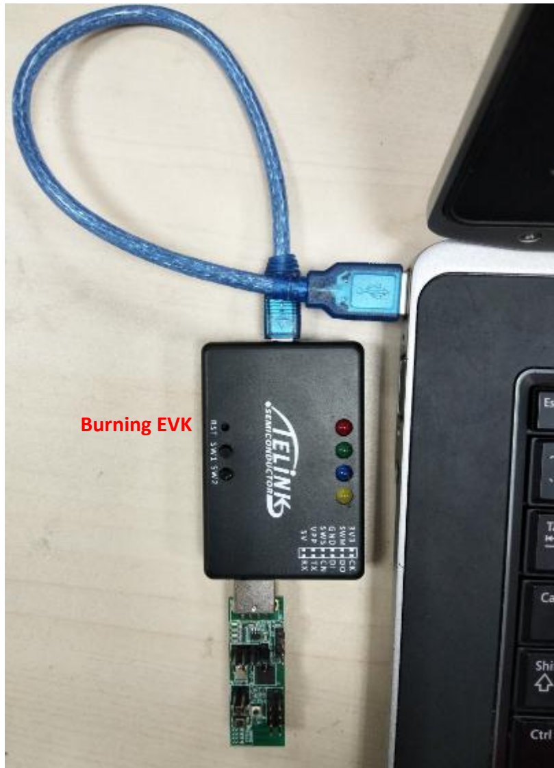
Figure 3 Connect EVK, Dongle and PC
