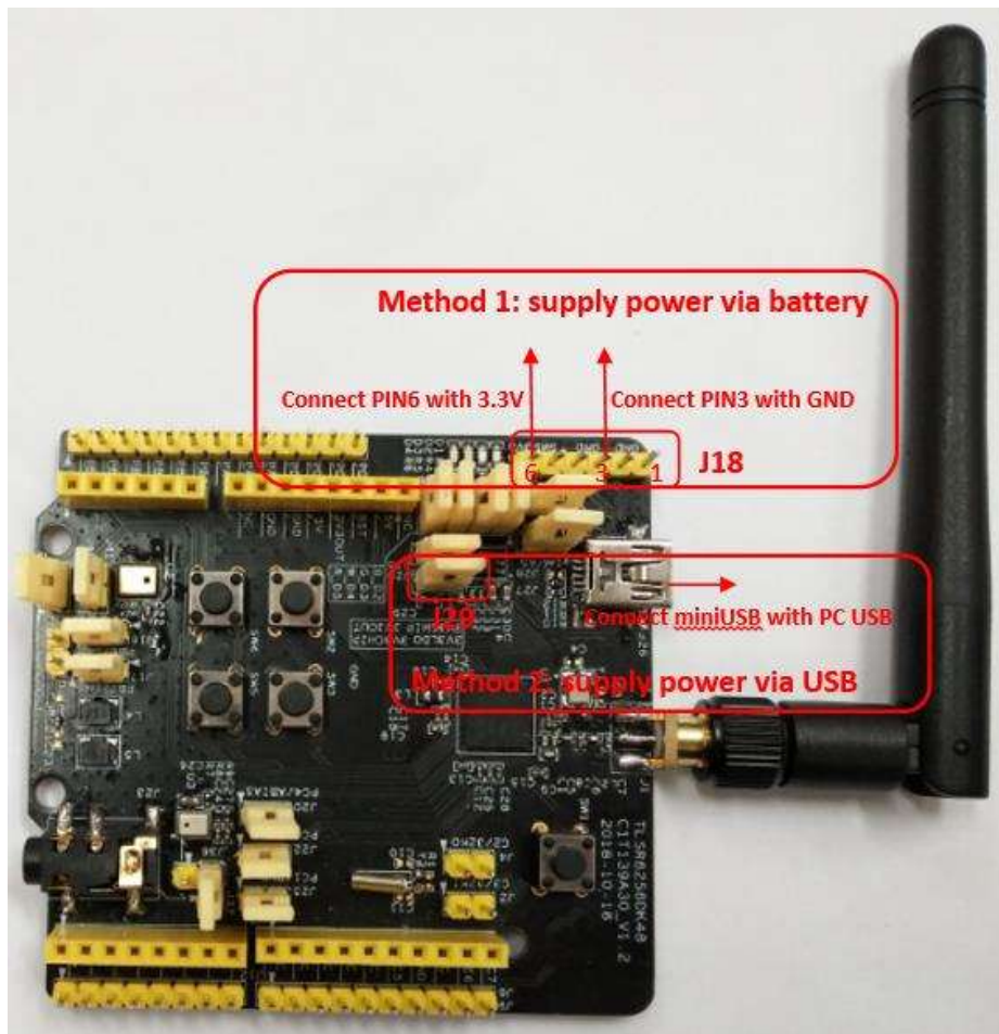
Figure 6 Connection chart to supply power
