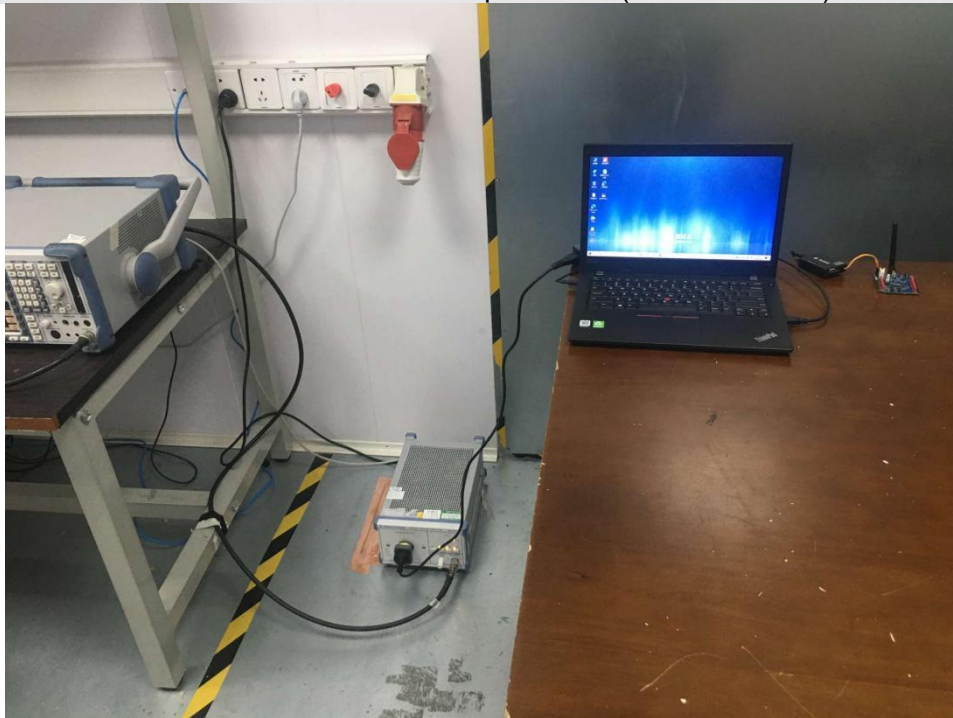
Conducted emissions at AC power line (150kHz-30MHz)
