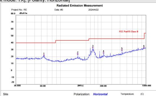
Limit: FCC Part15 Class B EUT: TLSR8208EDK56D M/N: TLSR8208EDK56D
