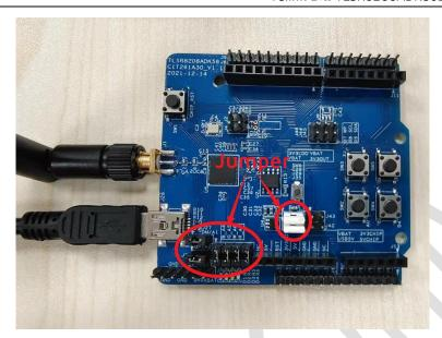
Figure 2-2 USB to LDO 3.3V power supply
