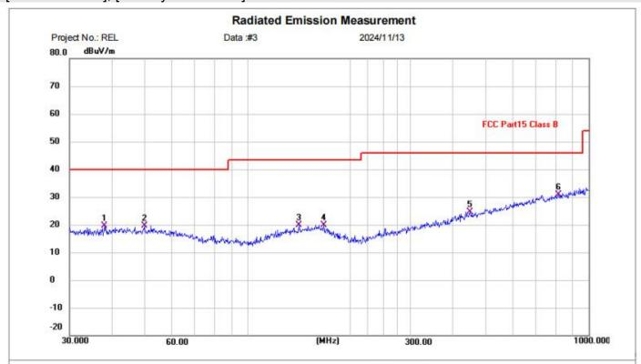
Site Polarization: Horizontal Temperature: (C)
