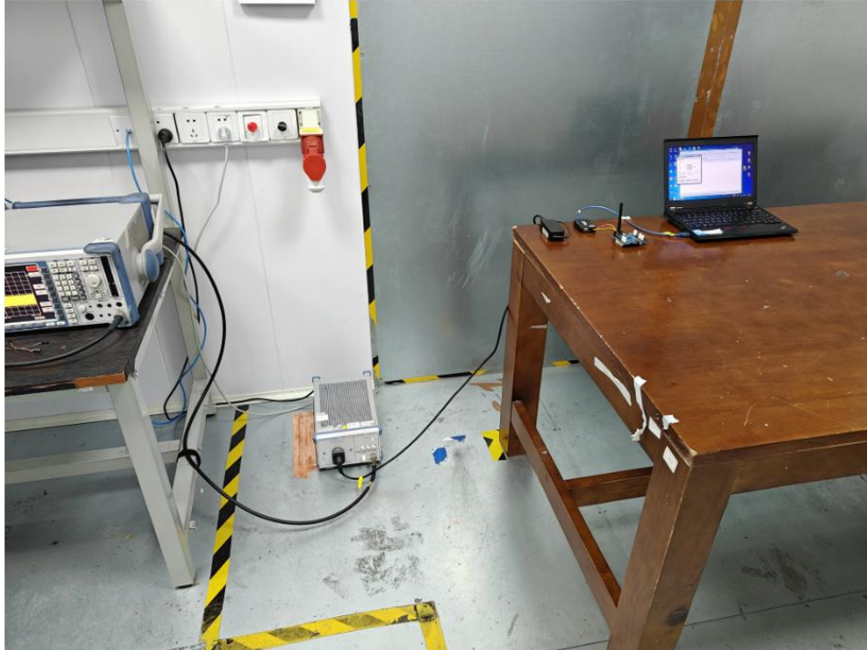
Conducted emissions at AC power line (150kHz-30MHz)
