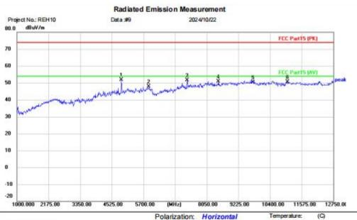
Site Limit: FCC Part15 (PK) EUT: TL3218X-DG64D M/N: TL3218X-DG64D Mode: BLE2M TX 2442
