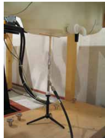
Photo of the dipole Antenna
