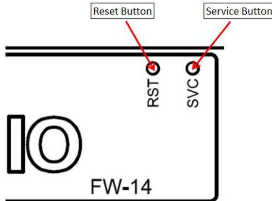
*Image shows the Reset button, Service button and also TXRX indicators.*
