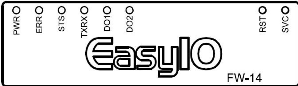
*Image shows the Status indicator, Error indicator and individual Digital Output indicator*
