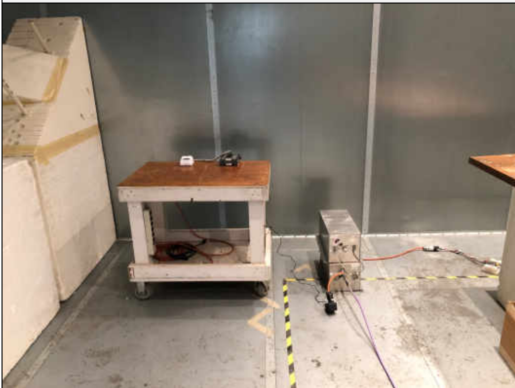
Test Setup for RF Conducted Emissions (AC Mains) – Using the FEC
