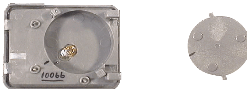
Figure 3: Installing the battery in the PID
