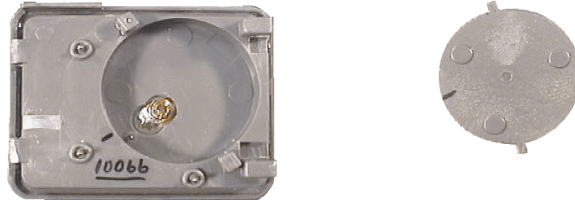
Figure 3: Installing the battery in the PID
