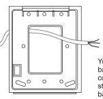
You should find that the backplate has holes for connection to most standard electrical backboxes.
