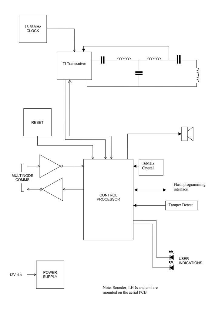
Figure 1: S831 Proximity Reader Block Diagram – Issue 2
