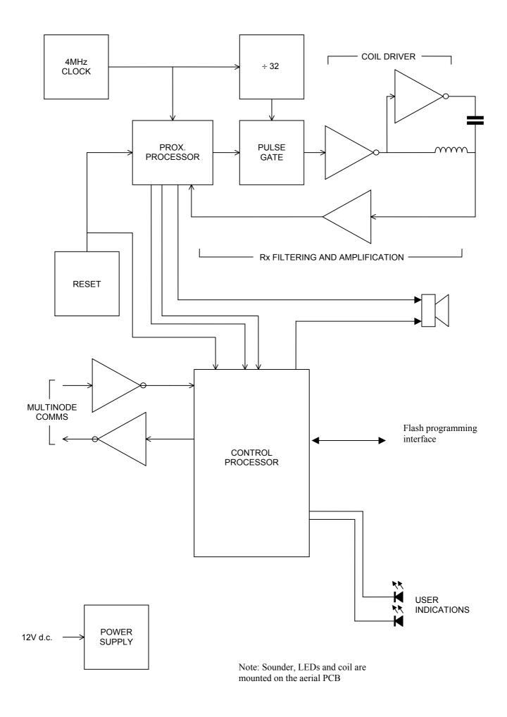
Figure 1: S830 Proximity Reader Block Diagram
