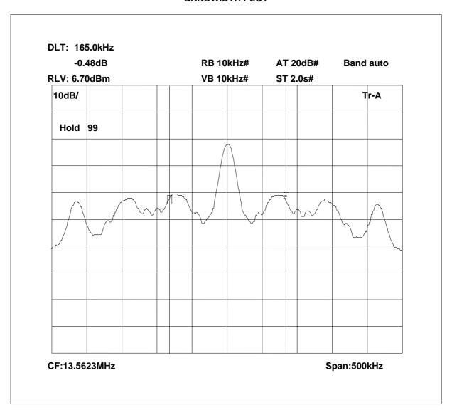
fl = 13.48130 MHz fh = 13.64630 MHz Occupied bandwidth = 165.0 kHz
