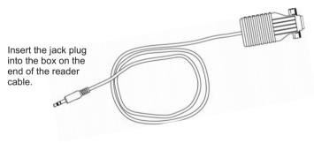
Connect to a serial port of a PC installed with the SMS software. Set up the port in the Install/Client Ports screen of the SMS software.
