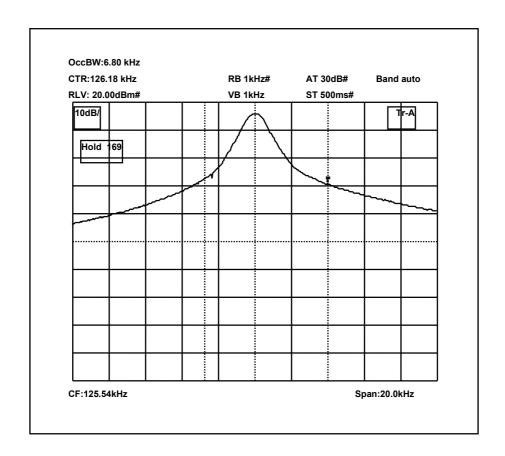
Occupied Bandwidth = 6.80 kHz FI = 122.760 kHz Fh = 129.560 kHz
