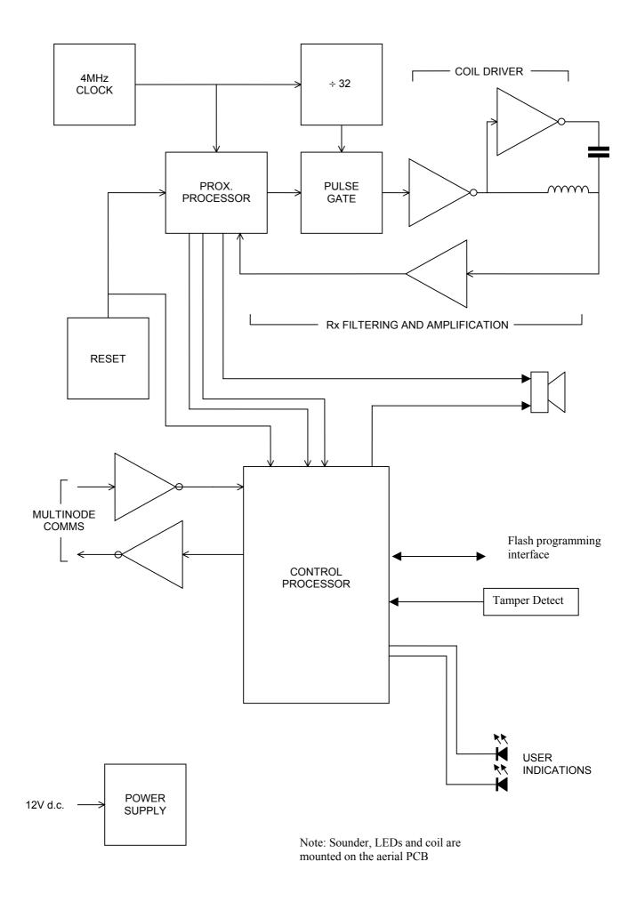
Figure 1: S820 Proximity Reader Block Diagram
