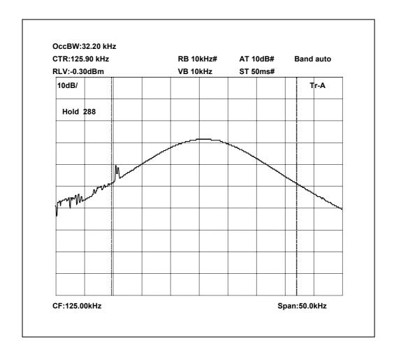
Bandwidth @-20dBc = 32.2kHz FI = 110.00kHz
