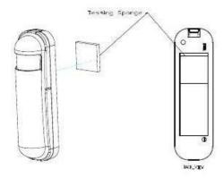
After finish the test and decide to fix, then you can remove tape A, and mounting the sensor by using tape B. The tamper key will pressed and let the sensor enter normal mode.
