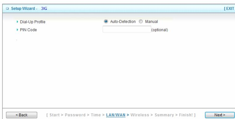
This screenshot shows the 'Setup Wizard - 3G' configuration page. It features options for Dial-Up Profile and PIN Code, with Auto-Detection selected. A note indicates '(optional)'. Navigation buttons at the bottom include '< Back', a breadcrumb trail ('Start > Password > Time > LAN/WAN > Wireless > Summary > Finish!'), and 'Next >'.
