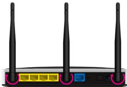
**Step 2:** Plug the RJ45 cable into LAN port 1~4 and connect with your PC or NB.
