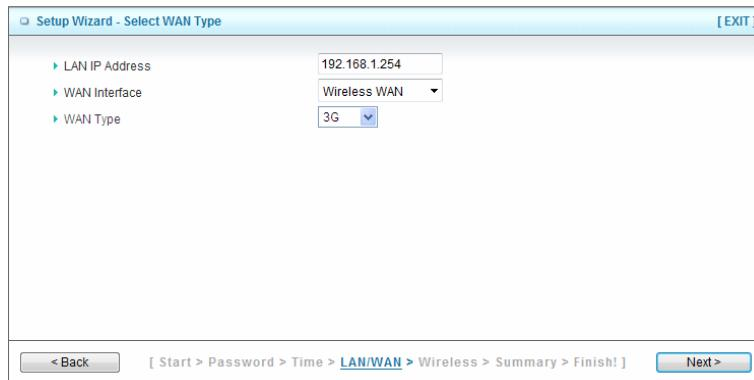
This screenshot shows the 'Setup Wizard - Select WAN Type' configuration page. It includes fields for LAN IP Address (192.168.1.254), WAN Interface (Wireless WAN), and WAN Type (3G). Navigation buttons at the bottom include '< Back', a breadcrumb trail ('Start > Password > Time > LAN/WAN > Wireless > Summary > Finish!'), and 'Next >'.
