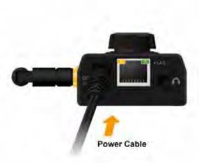
Once you have installed the Network Camera well and powered it on, the network accessing type LED will turn on. It means the system is booting up successfully. Furthermore, if you have a proper network connection, and access to the Network Camera, the LED will flash green under wired mode or orange under wireless mode.
