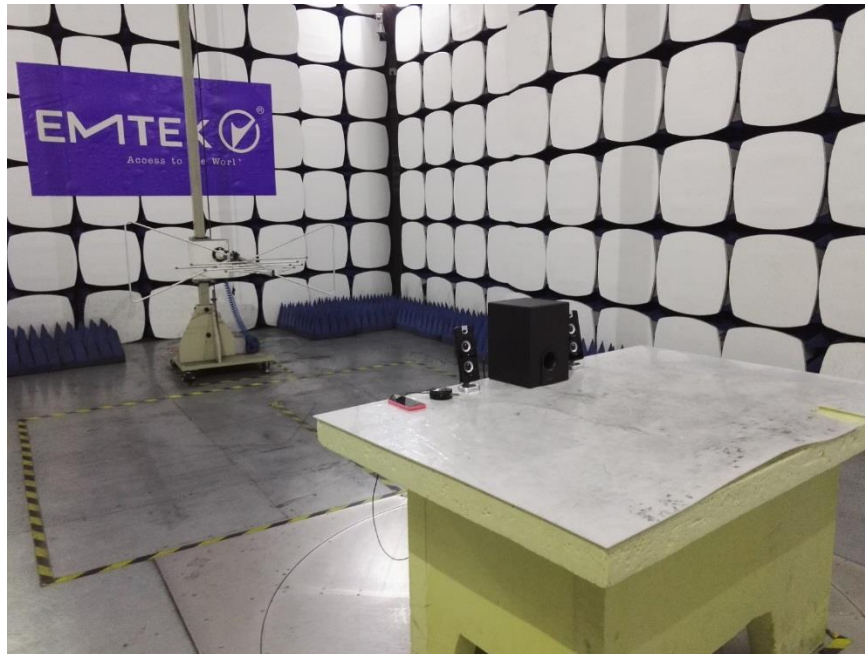
Set-up for Radiated Spurious Emission above 1GHz
