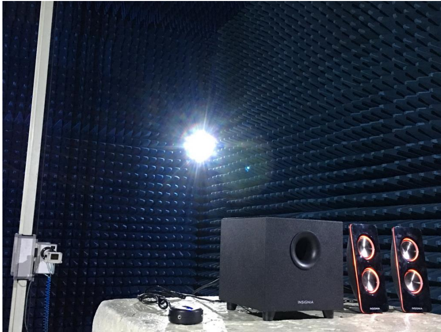
Photograph 5: Set-up for Radiated Spurious Emission, 18GHz - 26.5GHz
