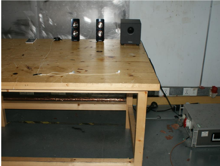
Photograph 1: Set-up for Conducted Emission on AC Mains
