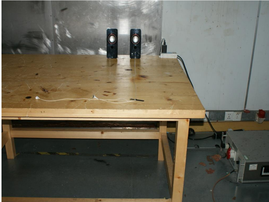
Photograph 1: Set-up for Conducted Emission on AC Mains
