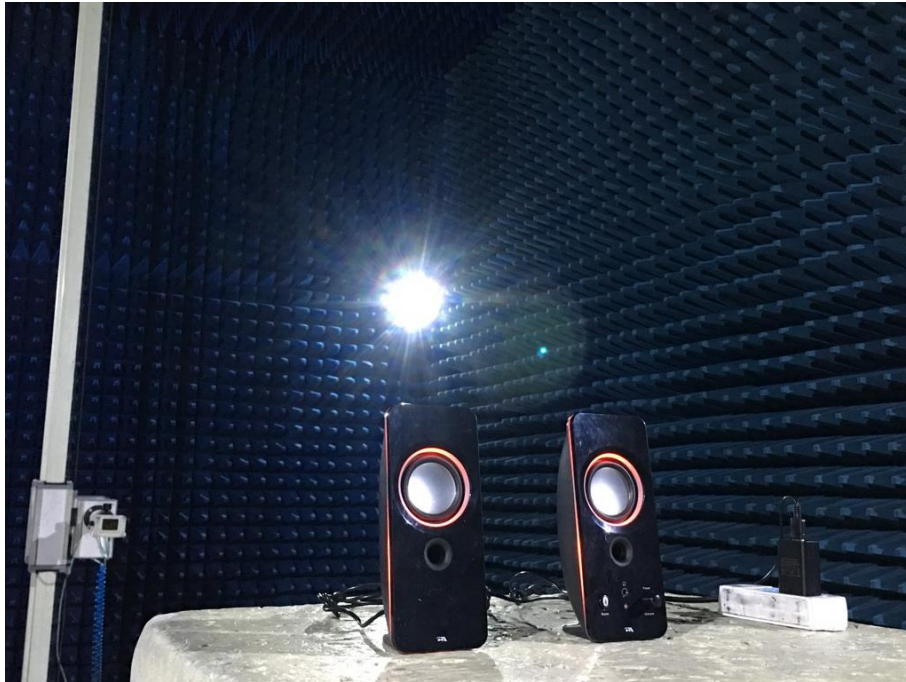
Photograph 5: Set-up for Radiated Spurious Emission, 18GHz - 26.5GHz
