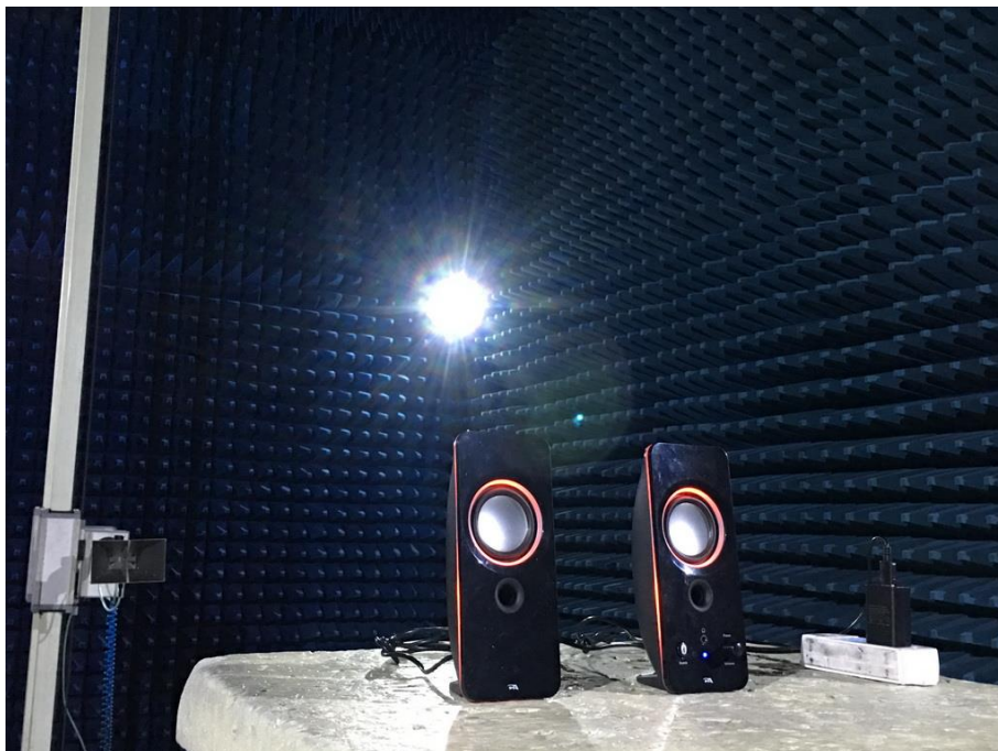
Photograph 4: Set-up for Radiated Spurious Emission, 1GHz - 18GHz
