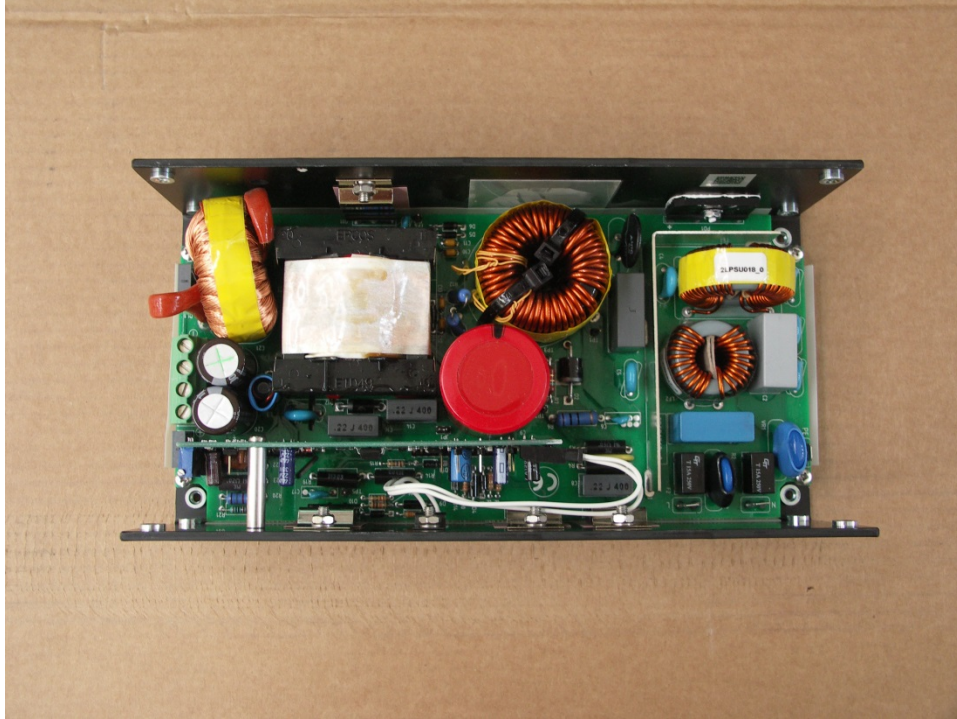
MAIN POWER SUPPLY
